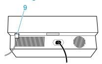
Use a standard network cable (RJ45 CAT.5E, to be ordered separately) to connect the network socket 9 and an Ethernet socket of the network.
