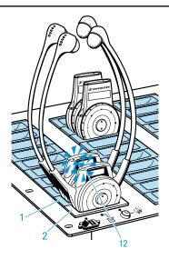
▶ Place the receiver into any charging compartment. The LED 12 on the receiver indicates the charge status.
